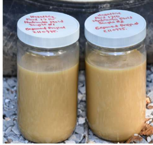
Figure 3. Photograph of a hydraulic fluid samples, shortly after collection from Plaintiff Hazeltine's Ford 1987 Ford 1710 tractor during the October 6, 2022, inspection. Notice the chocolate milk like appearance of the fluid, which is indicative of a fluid contamination issue. 37
